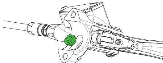
and alternately tighten the clamp bolts using the 4mm hex. Recommended tightening torque: **4-5 N.m**
